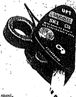
Sekuralt SK1 guided fall arrester device on semi-static rope, suitable for ropes ranging from Ø 10,5 to 13 mm. Thanks to its configuration, the fall-arrest device moves freely on the rope, and in case of fall, it will block immediately arresting the fall. Fixed device.
